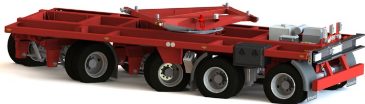
Adjustable bolster in all degrees of freedom for ensuring a smooth loading procedure.
