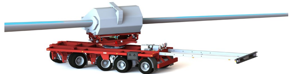
Extendable lighting support at the rear for reducing the rear rotor blade overhang.
