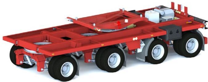
Manoeuvrable 4-axle trailing unit with high level of stability.
